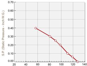
Air Flow (CFM - Cubic Feet Per Minute)
