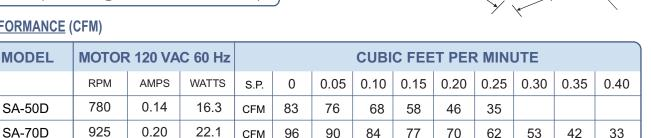
RPM (Revolution Per Minute) shown is nominal and performance is based on actual speed of test. Unit was tested with inlet grille, backdraft damper and outlet duct.
