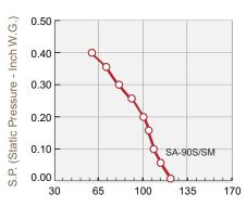
Air Flow (CFM - Cubic Feet Per Minute)
